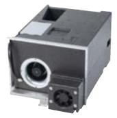
Complete encapsulation of the heatpump module ensures optimum heat insulation and reduces sound emissions to an unbeatable 63dB(A). Self-monitoring cooling offers protection against overheating up to an ambient temperature of 43°C.
